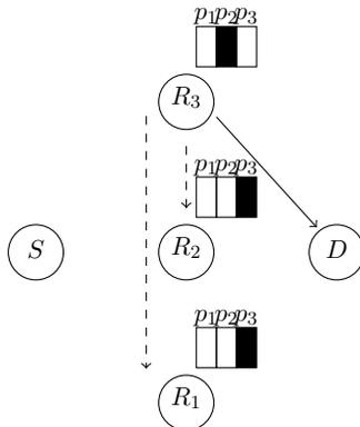
Figure 3: Example of the overhearing algorithm operation when three packets  $(p_1, p_2, p_3)$  have been transmitted through a wireless backhaul. Dark-shaded blocks indicate packets that are not available at a particular relay because they were lost during transmission from the source or MBS. Dashed lines denote overhearing.
