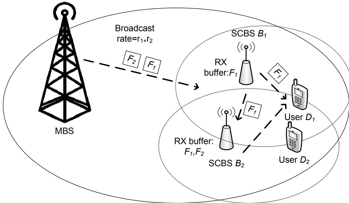
Figure 1: In the small-cell network topology adopted in this paper, each user receives a different video flow through the SCBS that is associated. In the wireless backhaul case both SCBSs can overhear packets from both video flows. The video flow  $F_1$  is depicted to avoid clogging the figure.
