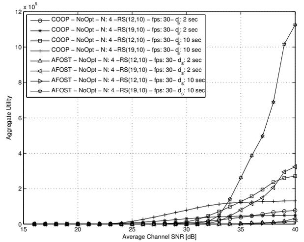
Fig. 4. Average utility vs. the channel SNR for 4 concurrently transmitting senders and without enabling utility optimization.  $d_s=2$  and 10 seconds while the frame rate is 30 fps.
