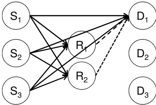
Fig. 1. The basic network scenario considered in this paper is cooperative unicast video transmission with the help of relay nodes  $R_1$  and  $R_2$ . Different line styles indicate transmission in a different time slot. In the case of multicast transmissions all the destinations are decoding all the video streams.
