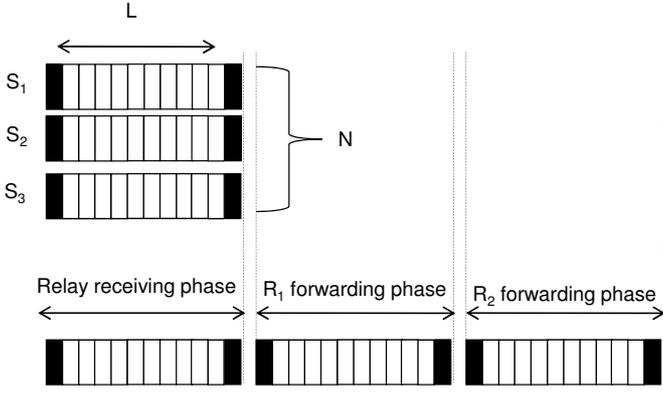
Fig. 2. The AFOST cooperative protocol for the simple topology with three senders. The dark-shaded blocks indicate the symbols that belong to the preambles and postambles of a packet and are used for channel estimation, while the non-shaded blocks are the symbols of the information packet.
