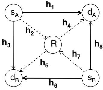
Fig. 1. Analog network coding of independent signal transmissions with the help of a random relay. The packet transmissions are received intentionally (thick solid lines) and unintentionally (narrow solid lines) at the destinations. Signal reception and forwarding at the relay is indicated with dashed lines.
