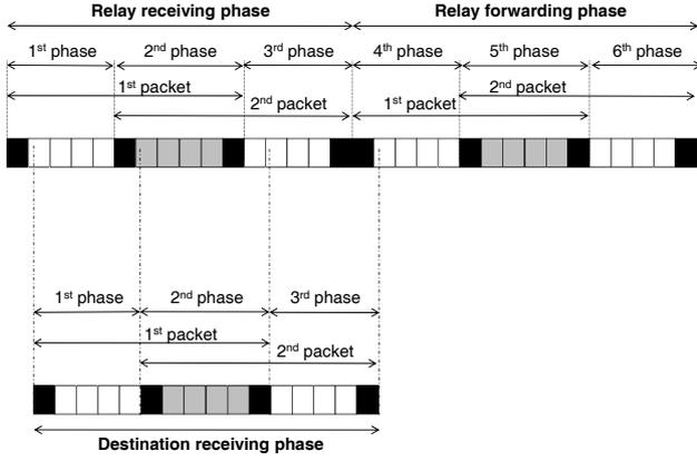
Fig. 2. Timing diagram of the 6-phase relaying used in the analysis. The grey-shaded areas indicate the portions of the packets (in terms of symbols) that are overlapped. The black-shaded areas indicate packet preambles and postambles that are used for channel estimation. Temporal difference in the received signals at the destination and the relay is also depicted.
