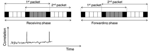
Fig. 4. Interfered/collided packets at the receivers and the relay visualized in terms of symbols. Correlation with the preamble spikes in the middle of the packet.
