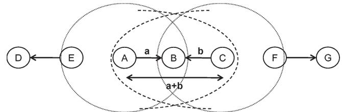
Fig. 1. Selection of a particular PHY transmission mode by nodes A and B may determine whether they can reach each other directly or they need node B as a router. Solid lines in the topology graph indicate packet transmissions, while dashed lines indicate the transmission range of nodes A and C.
