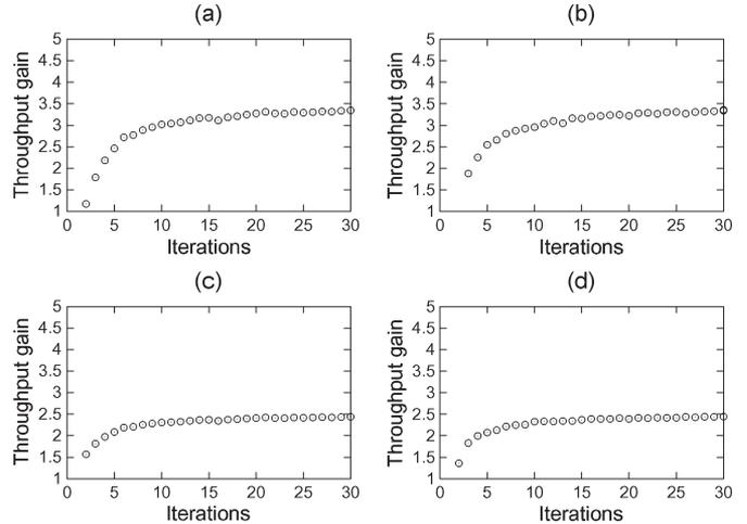
Fig. 10. Total throughput gain in the complete network versus the number of iterations of the cooperative algorithm. The term iterations refers to the number of invocations of the cooperative PHY rate-adaptation algorithm that are executed by a single node. Simulations are presented for different number/density of wireless nodes. (a) Nodes = 25, degree = 5. (b) Nodes = 50, degree = 5. (c) Nodes = 25, degree = 3. (d) Nodes = 50, degree = 3.
