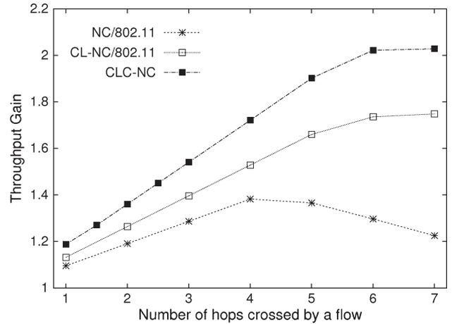
Fig. 7. Throughput gain for a different number of hops crossed by a flow. The percentage of multihop flows is 40%.
