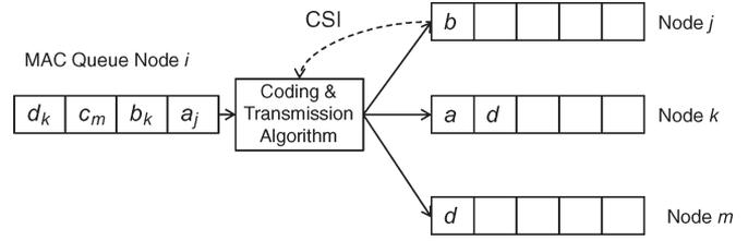
Fig. 4. Packet coding and transmission to multiple receivers. The introduction of a lightweight ACK mechanism of the link layer allows the optimization algorithm to evaluate faster the optimality of coding and scheduling decisions.
