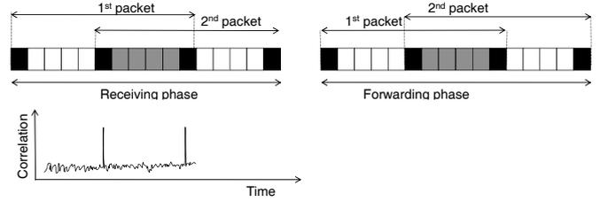
Fig. 3. Collided packets at the receivers and the relay in terms of symbols. Correlation with the preamble spikes when the preambles and postambles of two packets coincide.
