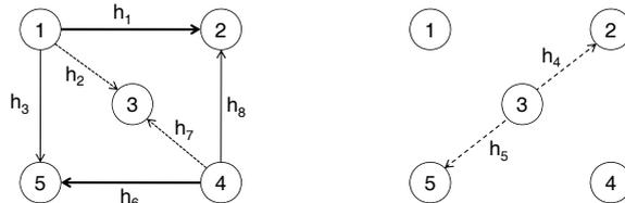
Fig. 1. Topology and signal analysis. Solid thick lines indicate the direct intended transmissions, while solid lines over channels  $h_3, h_8, h_2, h_7$  indicate the overheard packets. The left figure is the collision of two packets in the same time slot. In the right the relay forwards the locally collided packets.
