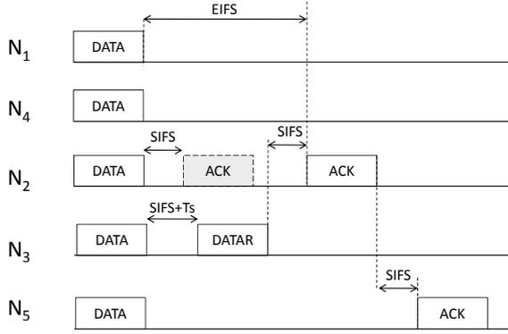
Fig. 2. Timing diagram of the distributed MAC protocol for the topology in Fig. 1. The dark-shaded ACK packet indicates the behavior in a successful direct transmission.
