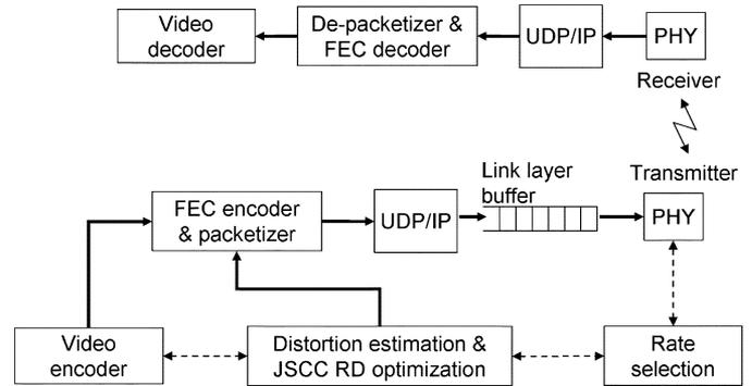
Fig. 2. Proposed cross-layer architecture for real-time video encoding and transmission in wireless LANs with adaptive PHY. Solid lines indicate data flow while dashed lines indicate cross-layer signaling.
