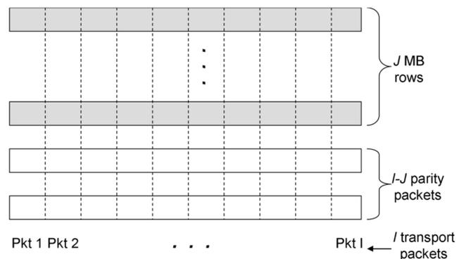
Fig. 3. Packetization with FEC across  $J$  source packets (MB rows). Each of the  $I$  transport packets can be encoded at a different PHY transmission rate  $r$ .
