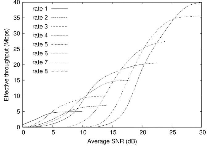
Fig. 4. Effective throughput versus channel SNR for all the different transmission rates of 802.11a and a multipath frequency-selective fading channel. Application payload is 2000 bytes.
