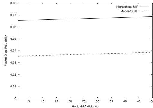
(b) Packet drop probability with respect to HA-GFA distance (Ch-GFA=25,  $T_f = 10$ )
