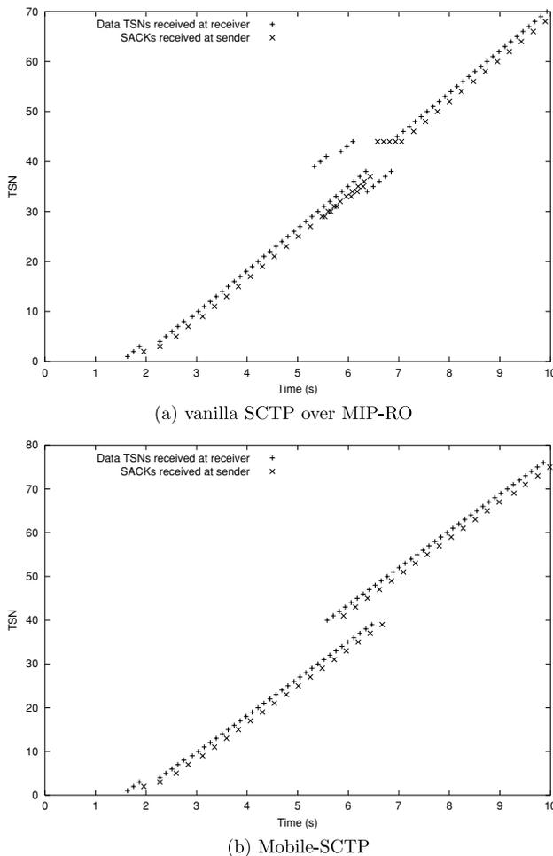
**Fig. 9** Sequence number progression uplink data flows in low bandwidth symmetric links. Data flow is on the uplink direction (MH → CH)
