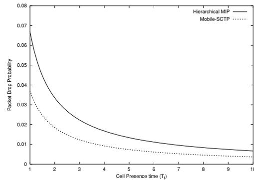
(a) Packet drop probability with respect to host cell presence time
