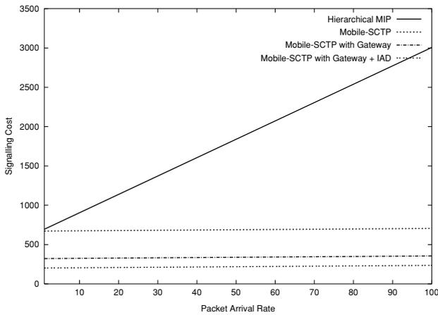
(a) Signalling cost with respect to packet arrival rate ( $T_f = 0.1$ )
