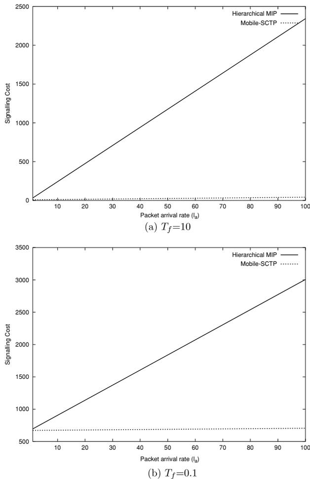
**Fig. 3** Signaling cost for fixed two values of MH residence time  $T_f$
