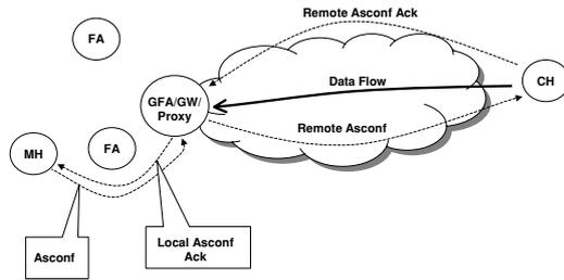
Fig. 5 Message exchange for Gateway/Proxy assisted handoff
