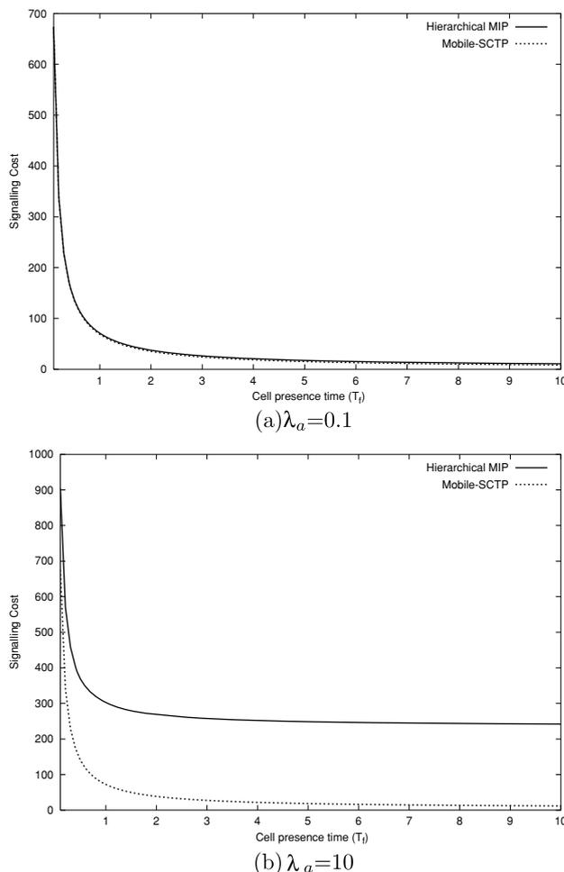
Fig. 2 Signalling cost for fixed packet arrival  $\lambda_a$
