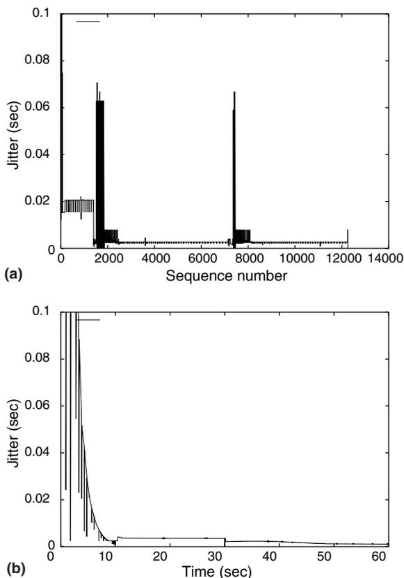
Fig. 9. Jitter for handoff experiment with CBR flows from a UMTS to WLAN 802.11b link. (a) Handoff from UMTS to WLAN with SCTP and (b) handoff from UMTS to WLAN with TFRC.
