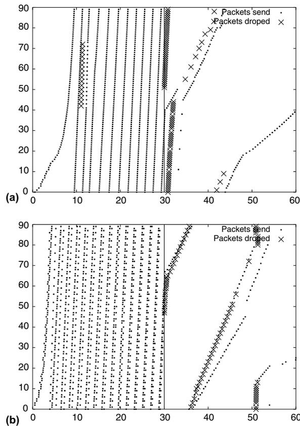
Fig. 7. Vertical handoff from UMTS to GPRS link. (a) Packet sequence numbers for TFRC and (b) packet sequence numbers for mobile-SCTP.
