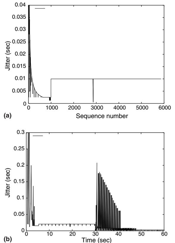
Fig. 10. Jitter for handoff experiment with CBR flows. (a) Handoff from UMTS to GPRS with TFRC and (b) handoff from WLAN to UMTS with SCTP.
