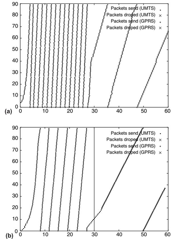
Fig. 8. Vertical handoff from UMTS to GPRS link with buffering. (a) Packet sequence numbers for mobile-SCTP and (b) packet sequence numbers for TFRC.
