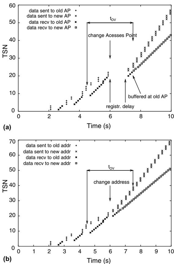
Fig. 5. Sequence number progression for downlink data flows in low bandwidth symmetric links. Host speed 20 m/s. (a) vanilla SCTP over MIP-RO and (b) mobile-SCTP.
