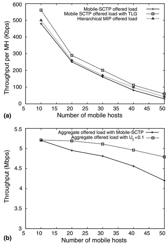
Fig. 4. Throughput for different handoff management protocols. (a) Throughput normalized per mobile host and (b) aggregate throughput.
