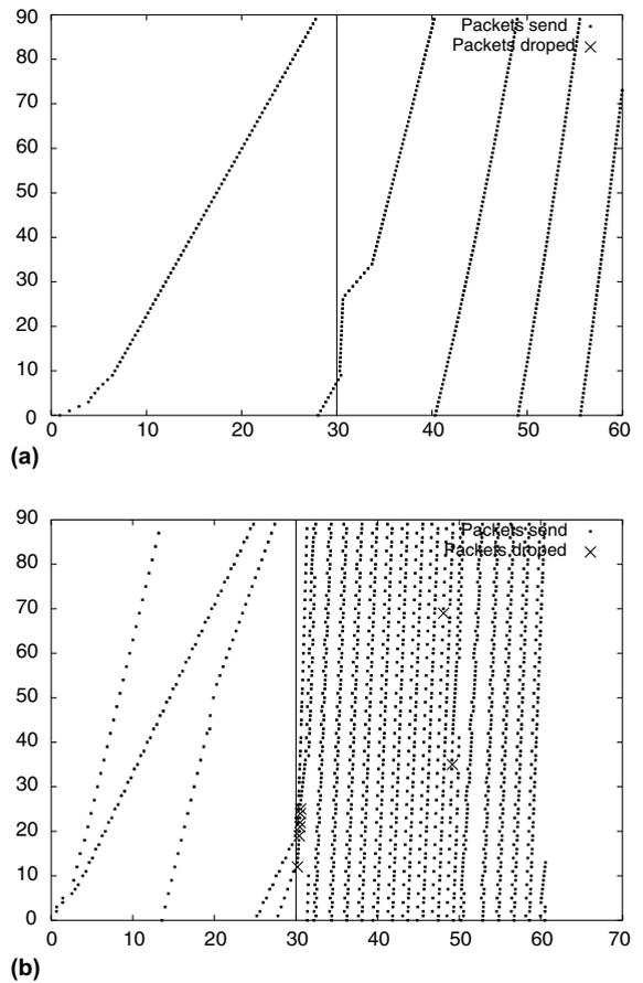
Fig. 6. Vertical handoff from GPRS to UMTS link. (a) Packet sequence numbers for TFRC and (b) packet sequence numbers for mobile-SCTP.
