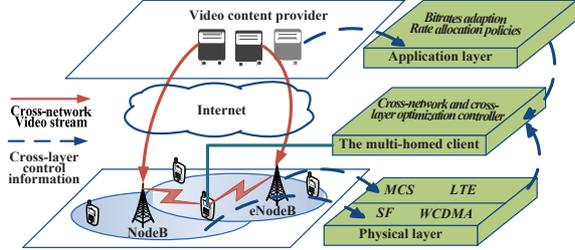
Fig. 1. The joint CNCL video streaming optimization scheme.
