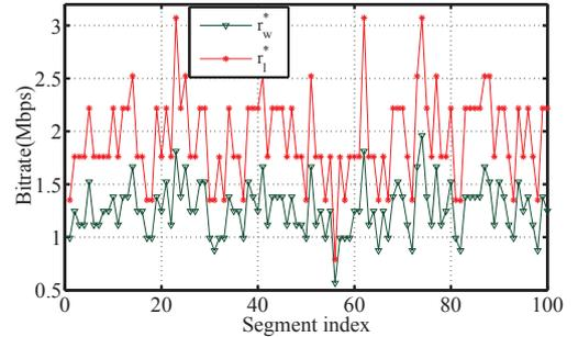
Fig. 2. The optimal bit-rate allocation curves with increasing segment number for the video sequence of *Shield* with the condition of  $\bar{\gamma} = 4dB$ .
