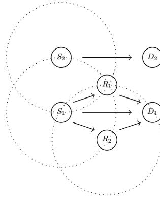
Fig. 1. Sources nodes  $S_1$  and  $S_2$  transmit simultaneously. Node  $R_1$  receives the interfering signal from the two sources and forward it to  $D_1, D_2$ . The dashed lines depict the transmission range of the respective nodes.
