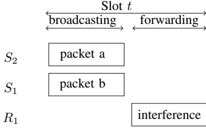
Fig. 2. Cooperative protocol for one slot. Each slot is separated in two phases.
