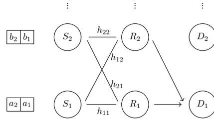
Fig. 2. Fundamental two-hop topology that includes multiple sources, relays and destinations. In the sample packets depicted on the left of the figure each source transmits two symbols successively. Any equal number of sources and relays can be supported by the system model.
