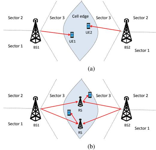
Fig. 1. (a) In LTE ICIC allows the BSs to coordinate the transmissions towards their respective destinations. (b) Application scenario of the proposed scheme in a cellular network where the two BSs transmit simultaneously towards their destinations in the same resource block. The relay nodes transmit in the next slot.
