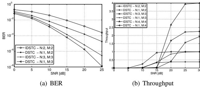
Fig. 3. Results for different number of sources  $N$  and all  $|h_{x,y}| = 1$ .
