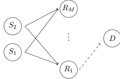
Fig. 1. Network model. The two sources  $S_1$  and  $S_2$  transmit simultaneously and the signals interfere at the relays. The relay selection policies investigated in this paper are responsible for identifying the relay that must forward its signal in order to improve interference cancellation at  $D$ .
