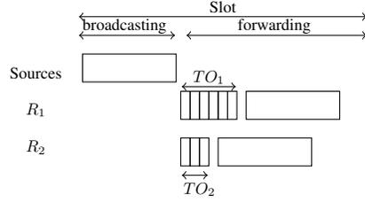
Fig. 2. Channel access from the relays based on a timer.
