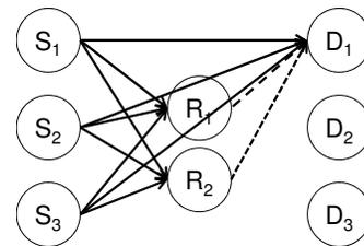
Fig. 1. Example network model with three simultaneously transmitting sources and two relays. Each source has one designated destination. Solid lines indicate transmissions during the broadcast phases. Dashed lines indicate transmissions in different forwarding phases.
