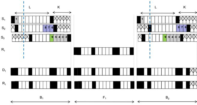
Fig. 2. Example of packet transmissions from two sources and one relay with ACMA. The dark-shaded blocks indicate the symbols that belong to the preambles and postambles of a packet. The blocks with an internal X indicate the empty symbol slots. The vertical dashed lines depict the fourth symbol slot where misalignment can occur but only in different broadcast phases.
