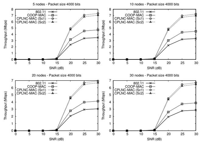
Fig. 4. Simulation results of the aggregate network throughput for different channel conditions and different number of nodes. Packet size of 4000 bits is used.
