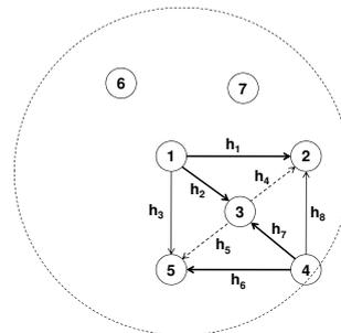
Fig. 1. Ad hop network topology that demonstrates physical layer network coding with cooperative relaying through node  $N_3$ . The solid lines indicate the concurrent broadcasting of packets from  $N_1$  and  $N_4$ , while the dashed lines indicate the forwarded mixed packet from  $N_3$ .
