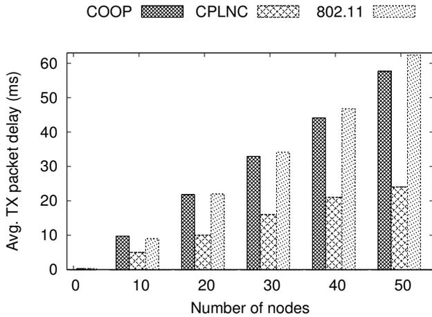
Fig. 5. Channel access delay for the three protocols under test.
