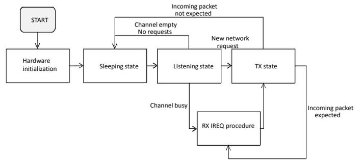
Fig. 2. Generic view of the state machine and interactions with the receiver interrupt service routine (RX\_IRQ).
