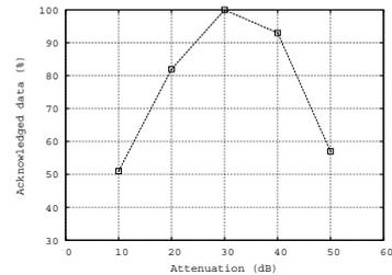
Fig. 7. Throughput vs. channel attenuation.
