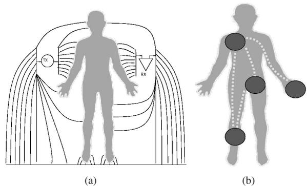
Fig. 1. Body-coupled communication consists of modulating capacitively induced electric fields through the human body (a), while our system model considers multiple on-body sensor nodes (b).
