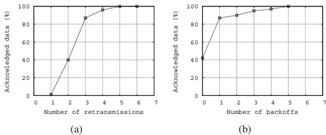
Fig. 6. Throughput vs. the allowed number of retransmissions and backoffs.
