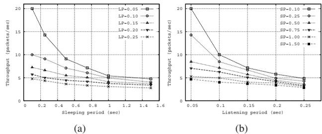
Fig. 5. Throughput vs. the SP and LP for different LPs and SPs respectively.
