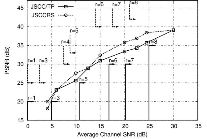
**Fig. 2.** Average PSNR of the Foreman sequence for JSCCRS and JSCC/TP with a multipath fading wireless channel model. Target frame rate is 30 fps.
