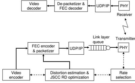
**Fig. 1.** The proposed cross-layer system for real-time video encoding and transmission in WLANs with adaptive PHY.
